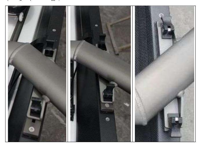
The underside of the plates have grooves cut into them to exactly match the round ends of the bolts. This ensures that when the cams are locked, the rigger cannot slide off. If the cams will not lock with moderate force, the rigger is not in the correct position.
