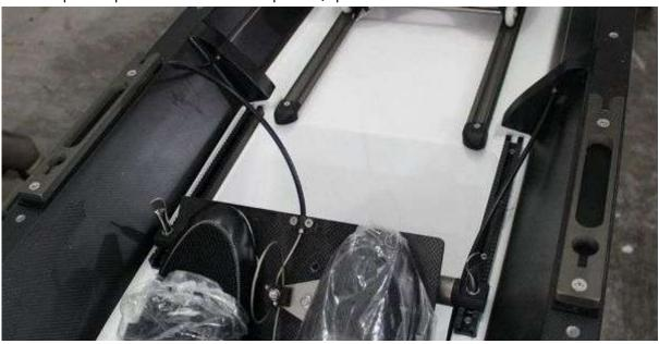
Next the cam needs to be attached to the rigger. Separate the cam parts, push the square necked bolt up through the square hole in the rigger foot, then put the spacer on to the rigger foot. Finally, hold the cam in place on the square necked bolt, and pass the small screw through the holes in the cam and the bolt. One point to note is that on one side of the cam are the symbols "—" and "+". With a set of brand new parts, make sure that the "—" is to the side that the cam will be pushed down.
