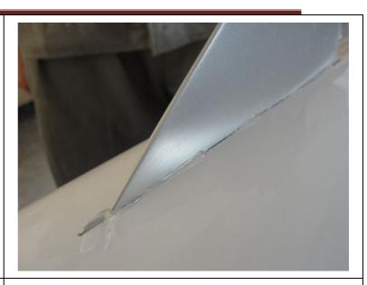
**Step 3**Push the back end of the fin down into the fin box.
