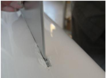
**Step 4**Use the piece of wood to move the fin towards the stern.
